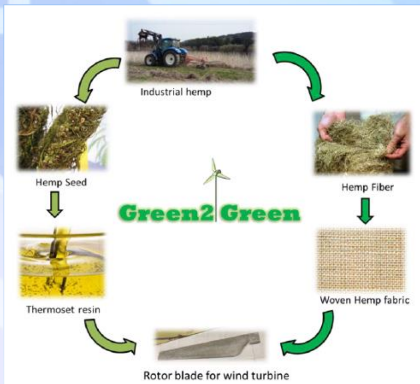
Figure2: Overview of obtaining renewable small wind turbine blade from initial industrial hemp cultivation to final structural component.
